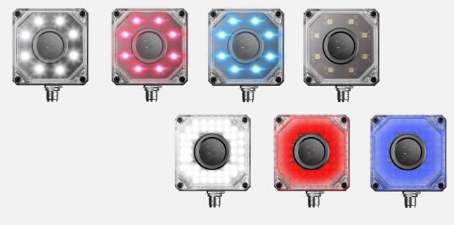
MV-SC2000-\*\* model light board is suitable for SC2000 series vision sensor, with a variety of types to be chosen from. You can select the appropriate type according to the site conditions to improve the imaging effect when testing the workpiece. The up, down, left and right light source on the board can be controlled individually, and support PWM to adjust the brightness to meet different requirements.
