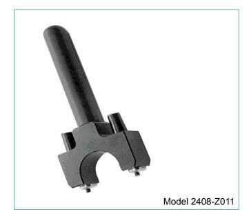
Electrode model 2408-Z011 for the surface resistance measurement according DIN 65181. The distance between the two electrodes is 50 mm.
