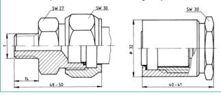
model 9945 Mating connector: Amphenol 62 GB-16F-10-6S Souriau 851-06E-C-10-6S or included in scope of delivery of model 8107 see dimensional drawing Dimensions: Weight: model 8103 40 g 100 g models 8106, 8107 IP67 Protection class: acc. to EN 60529 model 8103 models 8106, 8107 IP65
