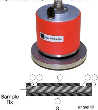
Depending on the connection wiring the RESISTOMAT<sup>®</sup> 2408 makes it possible to determinate the surface or volume resistance of the test sample.
